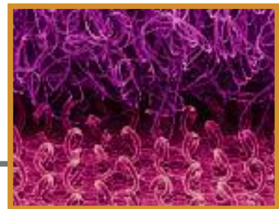
Colorized scanning electron micrographic image of joined VELCRO®. © Dee Breger, Drexel University
