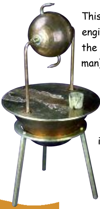
Heron's steam engine model by Karen Fisher courtesy of Smith College, History of Science and Technology Program
